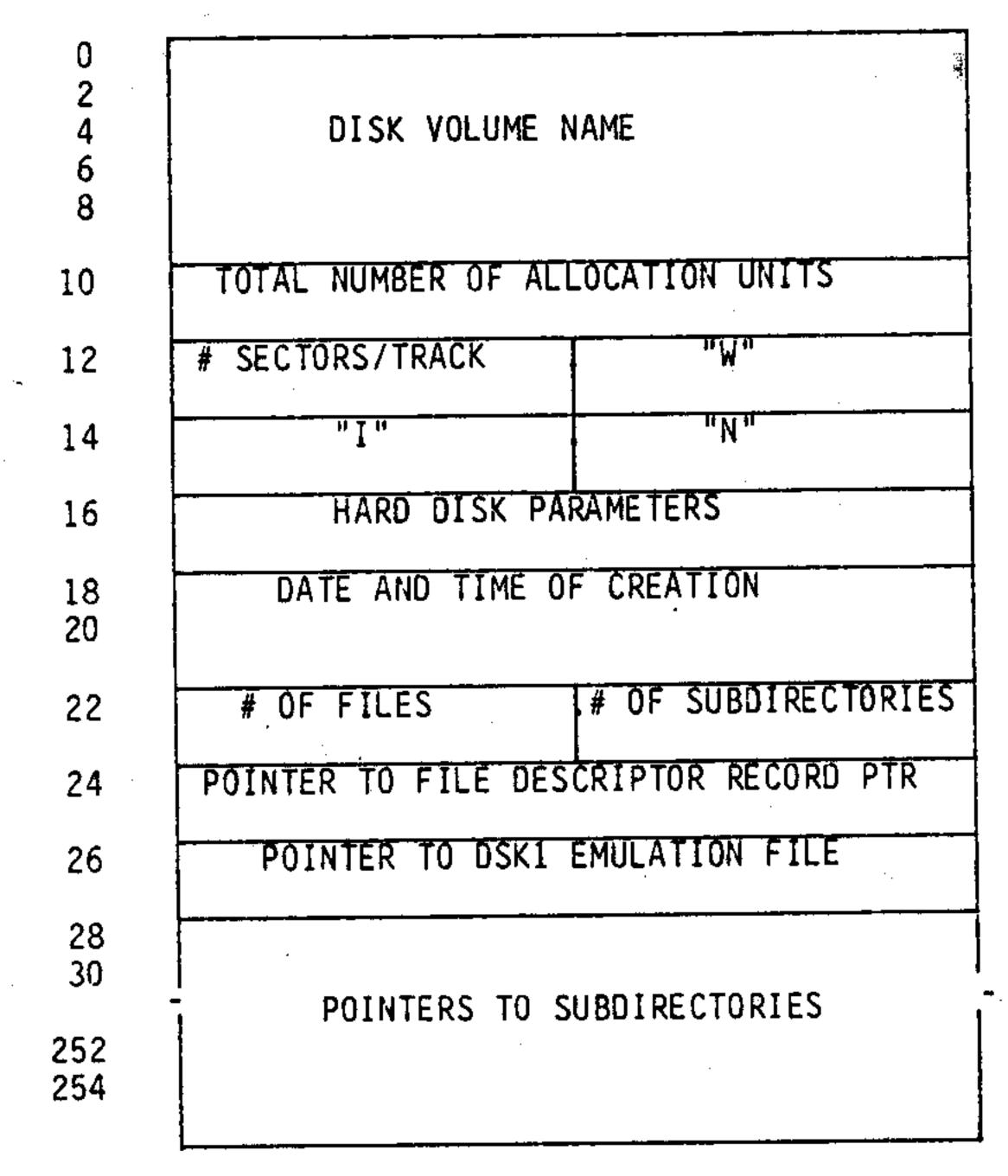
DISK VOLUME NAME - Contains the volume name of the hard disk. The volume name can be any combination of up to 10 ASCII characters, except for the space or period characters and the null character. The name is space filled to the right in the case of less than 10 characters.
